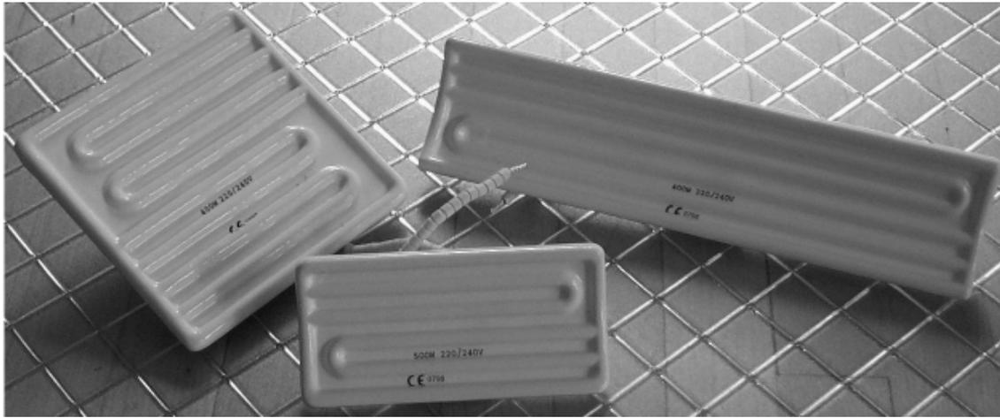
The Ceramic Heater is an efficient, robust heater which provides long wave infrared radiation. They are used in applications ranging from thermo-forming to pre-heating to paint curing. Nearly all materials to be heated or dried provide maximum absorption in the 3 - 10 microns range. The Ceramic Heater was developed with this fact in mind, and is the reason why they can be applied to such a diverse range of industrial processes.
