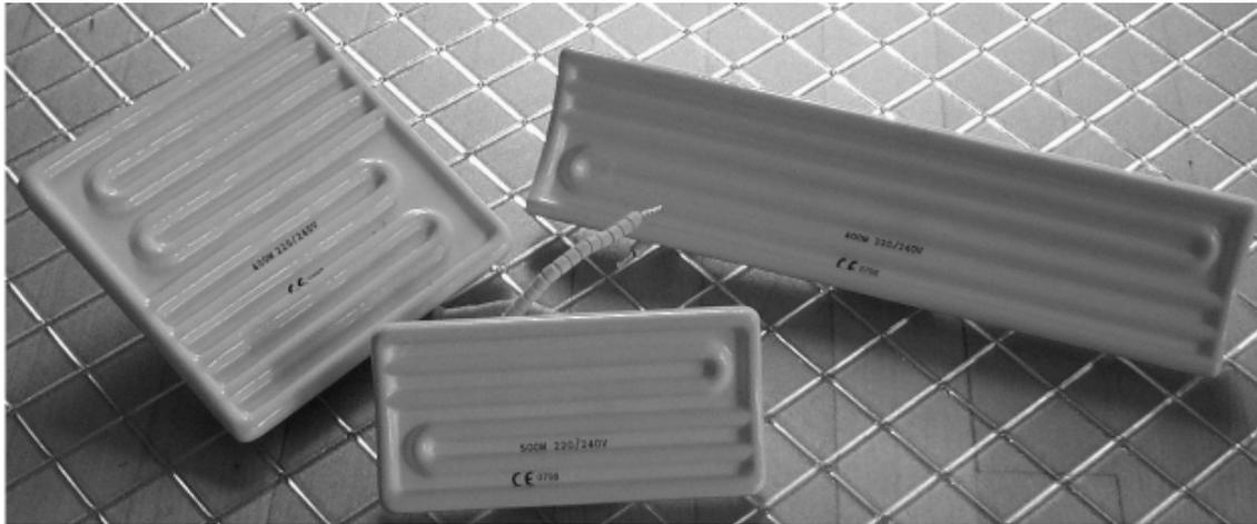
The Ceramic Heater is an efficient, robust heater which provides long wave infrared radiation. They are used in applications ranging from thermo-forming to pre-heating to paint curing. Nearly all materials to be heated or dried provide maximum absorption in the 3 - 10 microns range. The Ceramic Heater was developed with this fact in mind, and is the reason why they can be applied to such a diverse range of industrial processes.
